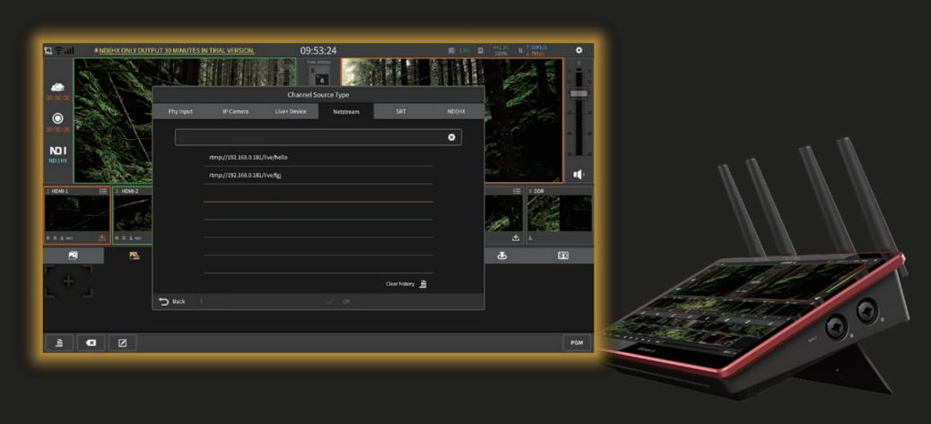
**NSCaster X2** has a 8-channel window and supports channel customization. You can select the input mode of various video sources such as physical camera input, IP camera input and network stream for each channel, which can meet various live streaming requirements.
